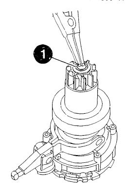
Disassembling overrunning-clutch drive
